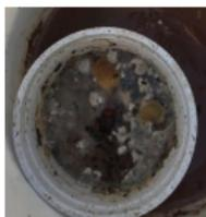
**Fig.7:** contaminated traditional trap after two weeks from setting
