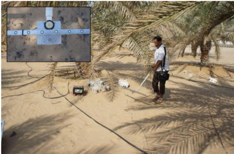
**Fig. 3.** Ahmed Al Muaini measuring the area of the shadow cast by date palm trees using the light stick. The inset show the details of the light sensors. There are 20 sensors on the stick.
