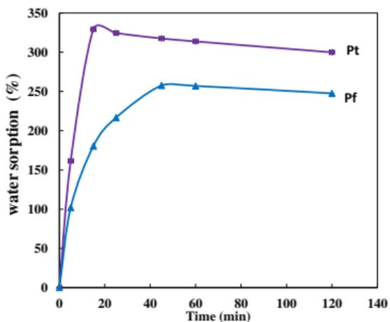
**Fig. 4.** Evolution of the water sorption for the marketed transplanting pellets (Pt) and the transplanting pellets produced from palm by product (Pf)
