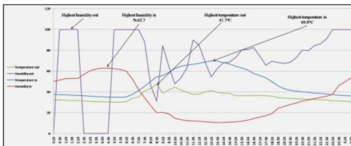
**Fig. 2.** Changes in temperature and humidity in and out of the PDH
